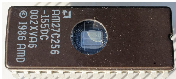
Figure 2: An AMI BIOS chip from a Dell 310, by Jud McCranie (CC BY-SA 4.0, 2018)
